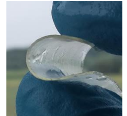
Photo-cured sample based on UrDMA1 and UrMA1 (50/50) before (up) and after immersion in water (down).
